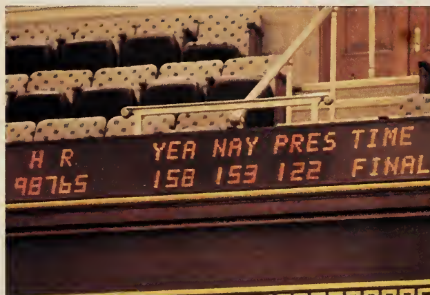
Located below the galleries on each side of the House Chamber, summary display panels present running tabulations as well as the time remaining for the vote in progress.
